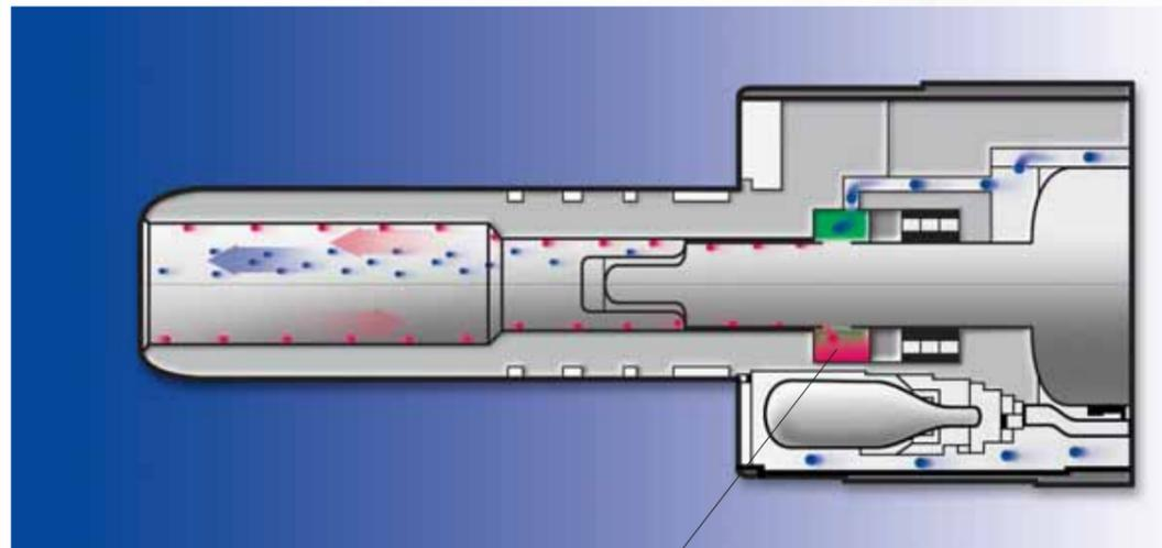
The KaVo Care-Ring protective barrier guards against contamination. All cleaning and care agents are trapped so that they do not reach the inside of the motor. And because the motor is not contaminated, its life is increased.
