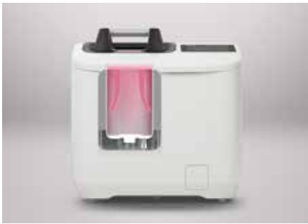
Sterilization and cooling 6. Heating up to 134 °C 7. Back-flush: Saturated steam is directed through the instruments 8. Sterilization: 3 min. at 134 °C 9. Cooling 10. The lid opens slightly 11. The lid can now be opened fully
